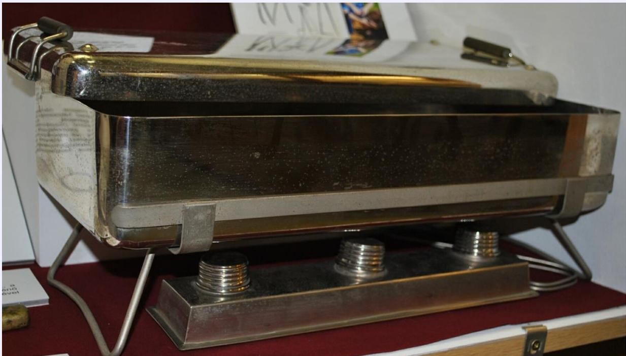
Autoclave for the disinfection of tools
